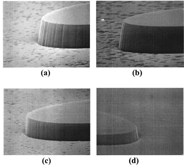
FIG. 5. SEM micrographs of GaN etch profiles; a conventional ICP configuration without the magnetic field (a) and no Kr (b), 10% Kr (c), and pure Kr (d) for a MICP configuration with the magnetic field; 10 mTorr, 80% Cl<sub>2</sub>/20% BCl<sub>3</sub> gas combination, 600 W inductive power, -200 V bias voltage, and 70 °C substrate temperature.
