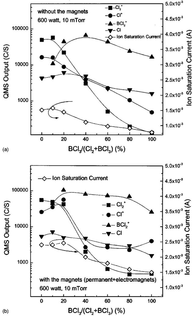
FIG. 2. Total positive ion saturation current measured by a Langmuir probe and QMS output intensities of Cl,  $Cl^+$ ,  $Cl_2^+$ , and  $BCl_2^+$  as a function of  $Cl_2/BCl_3$  at 10 mTorr and 600 W inductive power. Without the magnetic field (a) and with the magnetic field (permanent+electromagnets) (b).
