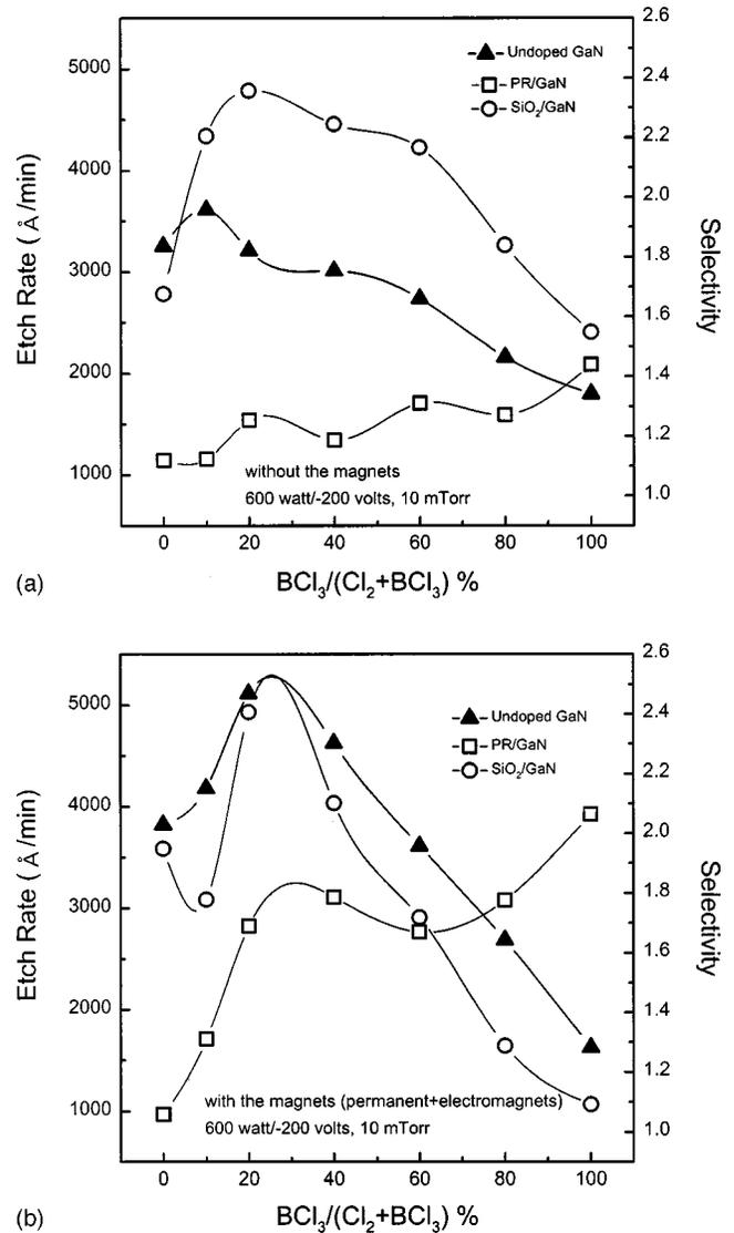
Fig. 1. GaN etch rates and selectivities as a function of gas combination of  $\text{Cl}_2/\text{BCl}_3$  plasmas at 10 mTorr, 600 W inductive power,  $-200$  V bias voltage, and  $70^\circ\text{C}$  substrate temperature. Without the magnetic field (a) and with the magnetic field (permanent+electromagnets) (b).
