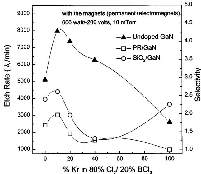
FIG. 4. GaN etch rate and selectivities as a function of Kr addition in the optimized Cl<sub>2</sub>/BCl<sub>3</sub> composition of 80% Cl<sub>2</sub>/20% BCl<sub>3</sub> with the magnets.
