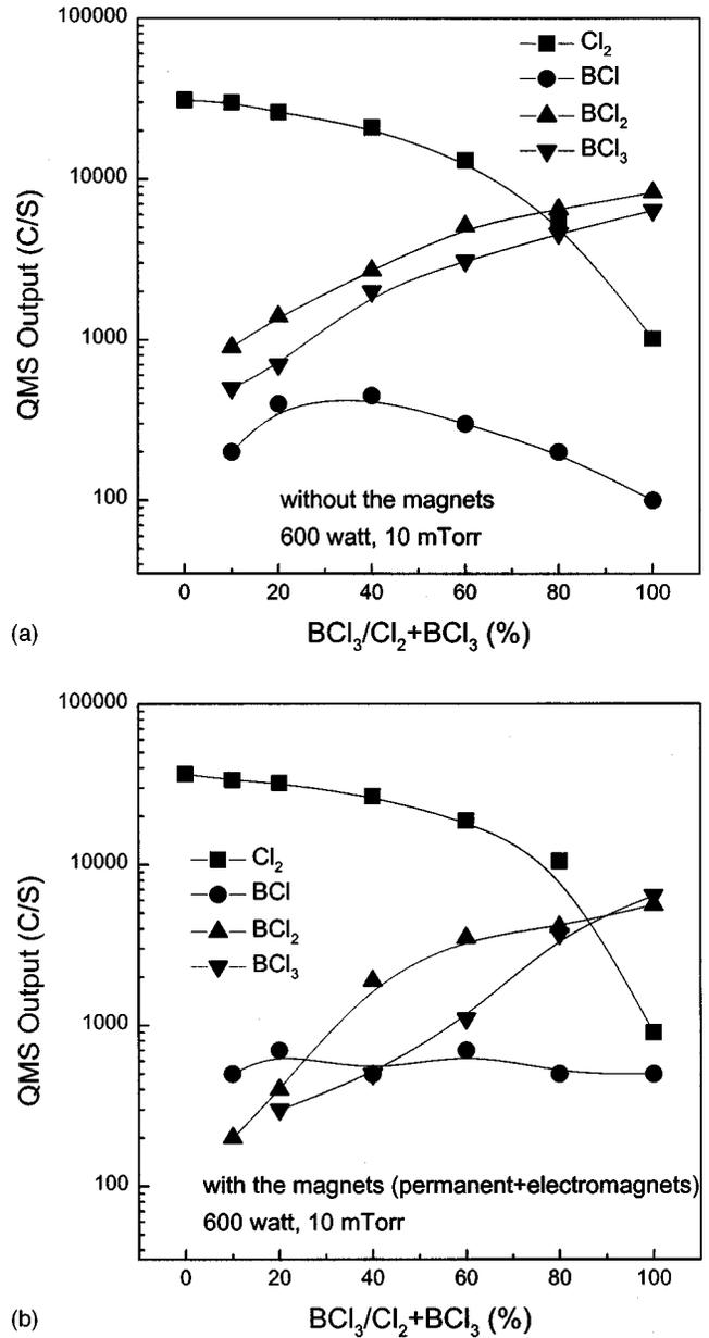
FIG. 3. QMS output intensities of neutral species such as  $Cl_2$ , BCl,  $BCl_2$ , and  $BCl_3$  as a function of gas combination of  $Cl_2/BCl_3$  plasmas at 10 mTorr and 600 W inductive power. Without the magnetic field (a) and with the magnetic field (permanent+electromagnets) (b).
